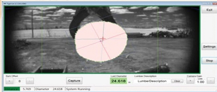
Fig.25 Vision system company Timber Diameter and length measurement using Infrared Technology
